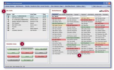
**Task Bar (Main Menu)** — All key calling functions are conveniently placed at the top of the screen and can be accessed through mouse commands, including Answer, Release, Hold/Resume, Transfer, Transfer to Vmail, Cancel Transfer, Park, Intercom, Page, Start/Stop Record, Options, Help, and Dial.
