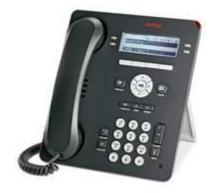
The 9504 Digital Deskphone is designed for light phone users with straightforward needs. It offers 12 administrable feature buttons, high-quality speakerphone, wired and wireless headset support, a context-sensitive interface, and a 4-way navigation cluster.
